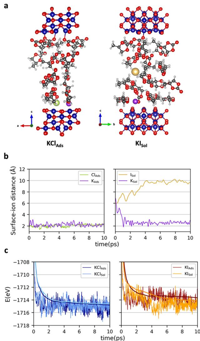
Fig. 2 (a) Representative snapshots of the most favorable  $\text{KCl}_{\text{Ads}}$  and  $\text{KI}_{\text{Sol}}$  AIMD simulations; variation along the AIMD simulation of the (b) surface–ion distance (K, Cl and I) at the most favorable conformation and (c) energy. Label code: Co (blue), O (red), C (black), H (white), K (purple), Cl (green), I (pale orange).
