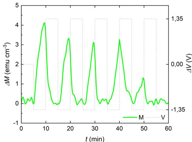
Fig. 6 Magneto-ionic cyclability of the 15 nm-thick cobalt oxide film in PC with  $2.5 \times 10^{-4}$  M KI under  $-1.35 \text{ V}/+1.35 \text{ V}$  voltage pulses of 10 min duration each, assessed from in-plane magnetic measurements while applying a magnetic field of 10 kOe.
