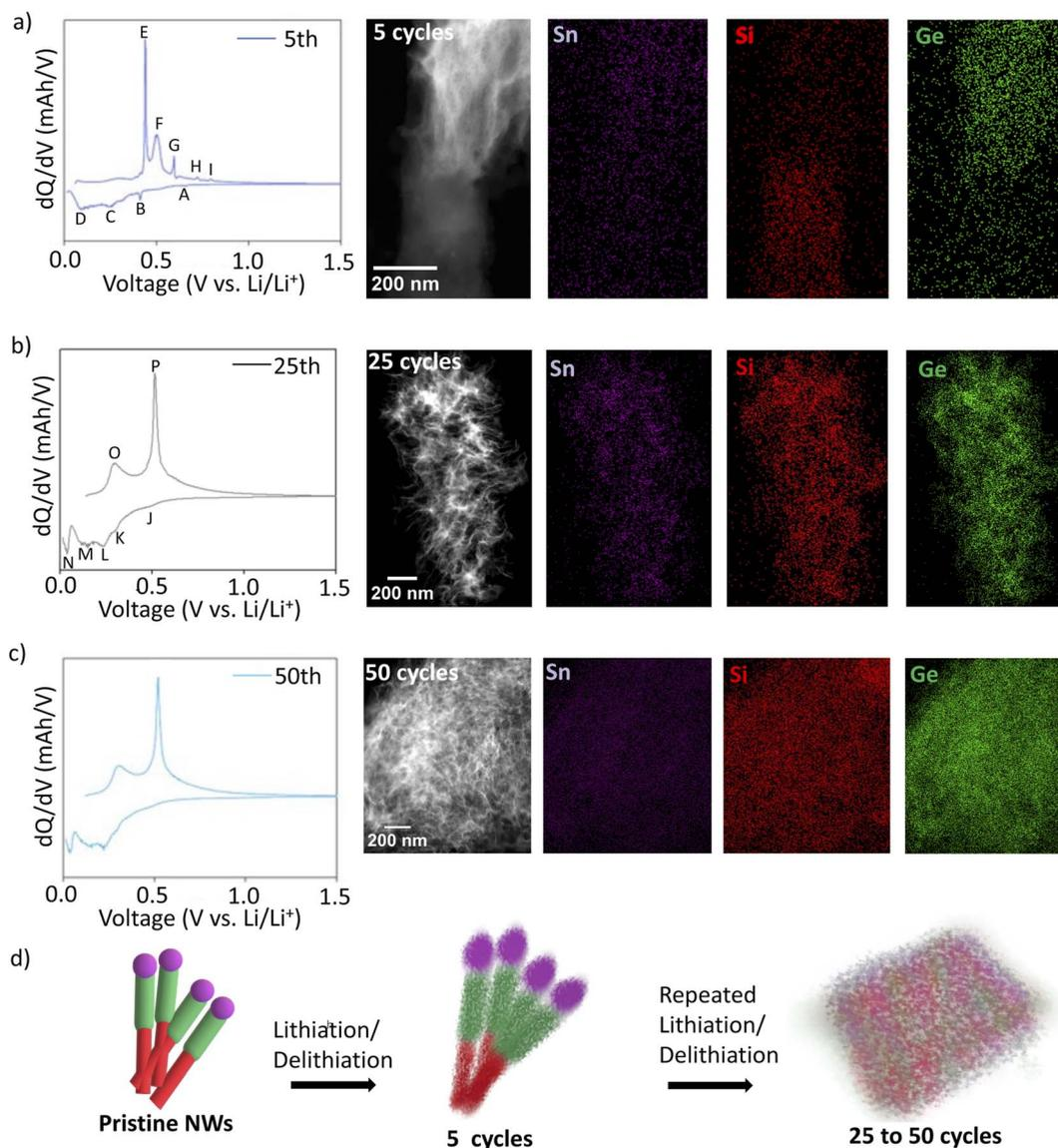
Fig. 4 Differential capacity plot of hSG NWs after (a) 5<sup>th</sup>, (b) 25<sup>th</sup> and (c) 50<sup>th</sup> cycle at 0.2C with corresponding STEM and EDX images. (d) Schematic illustration of the structural evolution of hSG NW during Li cycling.
