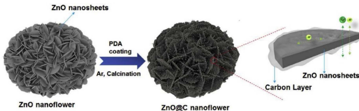
Scheme 7 Schematic illustration for the synthesis of ZnO@C nanoflowers. Reprinted with permission from ref. 320. Copyright © 2018 Elsevier B.V. All rights reserved.
