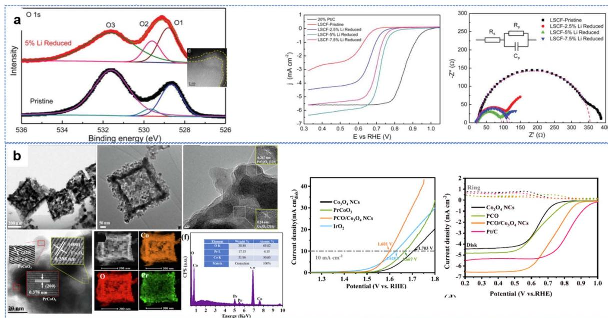
Fig. 12 Perovskites used for OER and ORR reactions: (a) Li reduced LSCF, (reproduced from ref. 211 with permission Copyright © 2018 Wiley-VCH) (b) P doped PCO/Co<sub>3</sub>O<sub>4</sub> heterojunction from ZIF-67. (Reproduced from ref. 214 with permission Copyright © 2022 Elsevier).
