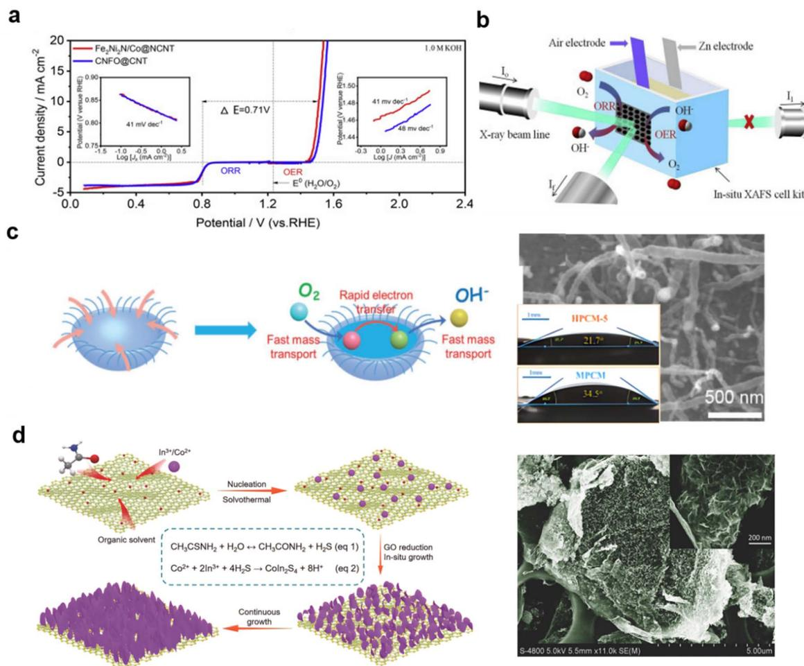
Fig. 17 Combining transition metal materials on CNTs with graphene: (a) and (b)  $\text{Fe}_2\text{Ni}_2\text{N}/\text{Co}@/\text{NCNT}$  with *in situ* XAFS for ZABs, (reproduced from ref. 280 with permission. Copyright © 2019 Elsevier) (c) jellyfish-like CNTs with Mott–Schottky junction, (reproduced from ref. 282 with permission Copyright © 2020 Wiley–VCH) (d) thiospinel  $\text{CoIn}_2\text{S}_4$  reduced on GO. (reproduced from ref. 284 with permission. Copyright © 2018 Wiley–VCH).
