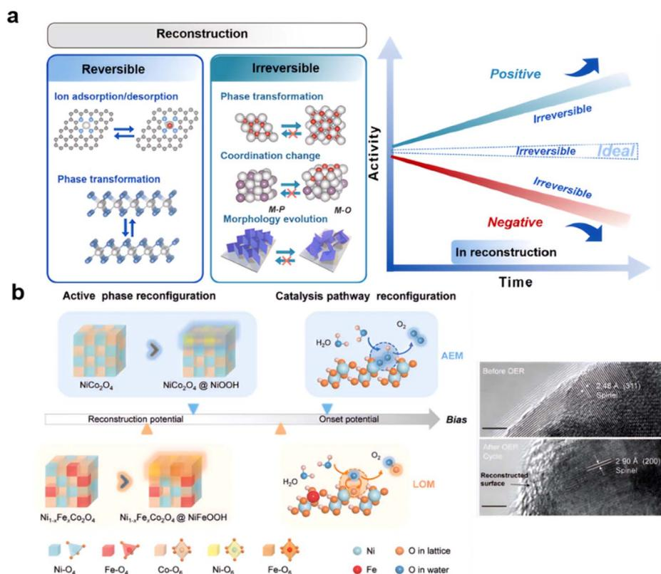
Fig. 19 (a) Diagram of different types of reconstruction and durability, (reproduced from ref. 294 with permission. Copyright © 2021 from John Wang *et al.*) (b) surface reconstruction of  $\text{NiCo}_2\text{O}_4$  and Fe doped  $\text{NiCo}_2\text{O}_4$ . (Reproduced from ref. 299 with permission. Copyright © 2022 Wiley-VCH).
