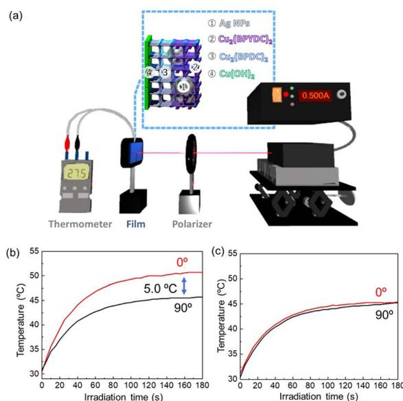
Fig. 6 (a) An experimental setup for the polarization-dependent plasmonic heating of the AgNPs@Cu<sub>2</sub>(BPYDC)<sub>2</sub>-on-Cu<sub>2</sub>(BPDC)<sub>2</sub> oriented film. Sample temperature as a function of laser irradiation time for (b) the oriented thin film and (c) the randomly oriented thin film.
