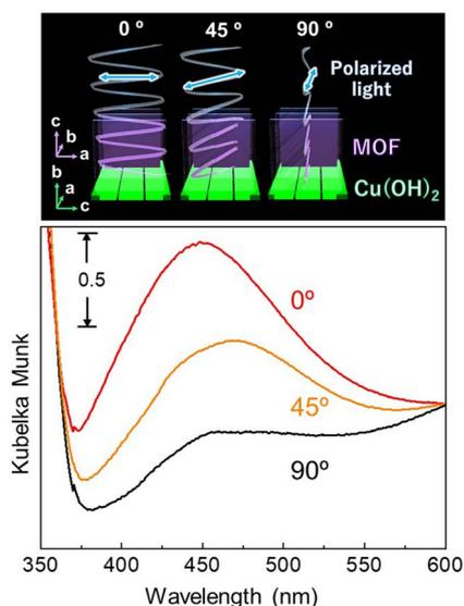
Fig. 5 Polarization-dependent UV/Vis reflection spectra of the AgNPs@Cu<sub>2</sub>(BPYDC)<sub>2</sub>-on-Cu<sub>2</sub>(BPDC)<sub>2</sub> thin film. Angles in the figure show the angles between the *a*-*c* plane of the MOF crystal and the electric field component of polarization of the light as described in the image above.
