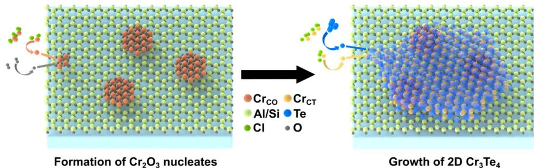
Fig. 4 A schematic diagram illustrating the proposed crystal growth model for epitaxially grown 2D  $\text{Cr}_3\text{Te}_4$  on the mica substrate. The process has two steps, with the first step being the formation of  $\text{Cr}_2\text{O}_3$  seed particles, and the second step being the growth of  $\text{Cr}_3\text{Te}_4$  based on  $\text{Cr}_2\text{O}_3/\text{Cr}_3\text{Te}_4$  interfaces.
