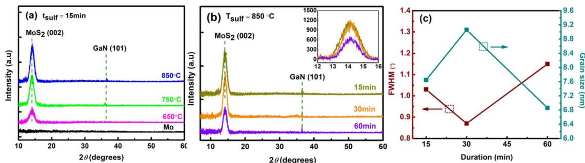
Fig. 4 (a) HR-XRD spectra of the MoS<sub>2</sub> films grown at different temperatures of 650 °C, 750 °C, and 850 °C for 15 min. (b) HR-XRD patterns of the 850 °C sample grown for different durations. (c) Full width at half maximum (FWHM) of the main XRD peak and the corresponding grain sizes of 850 °C sample as a function of sulfurization duration.
