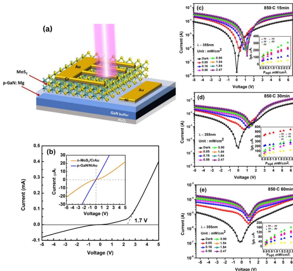
Fig. 5 (a) Schematic diagram of the n-MoS<sub>2</sub>/p-GaN heterojunction photodetector. (b) Dark  $I$ - $V$  curve of the n-MoS<sub>2</sub>/p-GaN heterojunction photodetector and the metal-semiconductor contact properties (inset). (c-e) Photoresponse of the n-MoS<sub>2</sub>/p-GaN heterojunction PD under varying light intensities. Inset shows the light intensity dependence of the photocurrent at different voltage biases.
