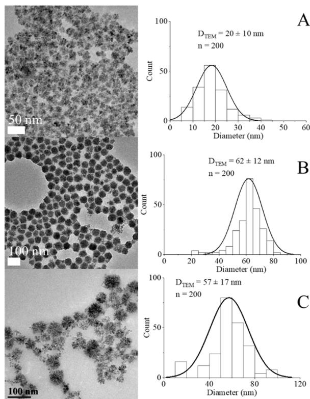
Fig. 3 TEM images and histograms for  $D_{\text{TEM}}$  of NFs prepared from  $[\text{Mn}(\text{acac})_3]/[\text{Fe}(\text{acac})_3]$  = (A) and (B) 1 & 3, respectively at 200 °C, (C) ratio = 7 at 250 °C.
