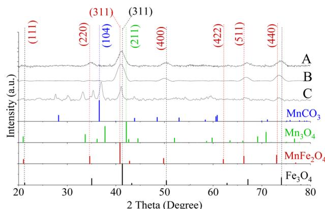
Fig. 4 XRD patterns of  $\text{Mn}_x\text{Fe}_{3-x}\text{O}_4$  NFs prepared from  $[\text{Mn}(\text{acac})_3]/[\text{Fe}(\text{acac})_3]$  ratio equal to (A) 1 and (B) 3 at 200 °C, (C) 7 at 250 °C. A secondary phase matched  $\text{MnCO}_3$  (Reference ICDD PDF card no. 00-044-1472) was found for NFs prepared from a precursor ratio equal to 7 at 250 °C. No detected peaks matched  $\text{Mn}_3\text{O}_4$  (PDF card no. 01-080-0382).
