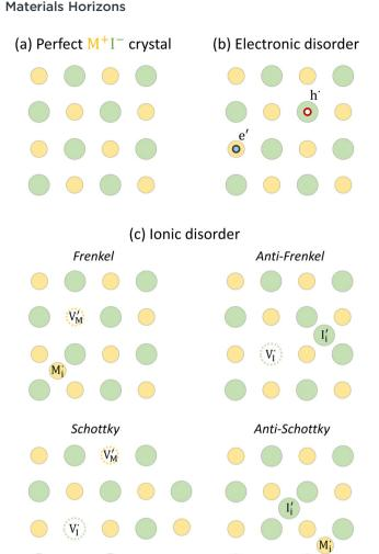
Fig. 1 (a) Perfect crystal of a square metal iodide lattice MI. (b) Electronic disorder involving electronic defects e' and h\*. (c) Different types of ionic disorder involving metal and iodide point defects (interstitials  $I_i'$  and  $M_i^{\bullet}$  and vacancies  $V_I^{\bullet}$  and  $V_M'$ ).
