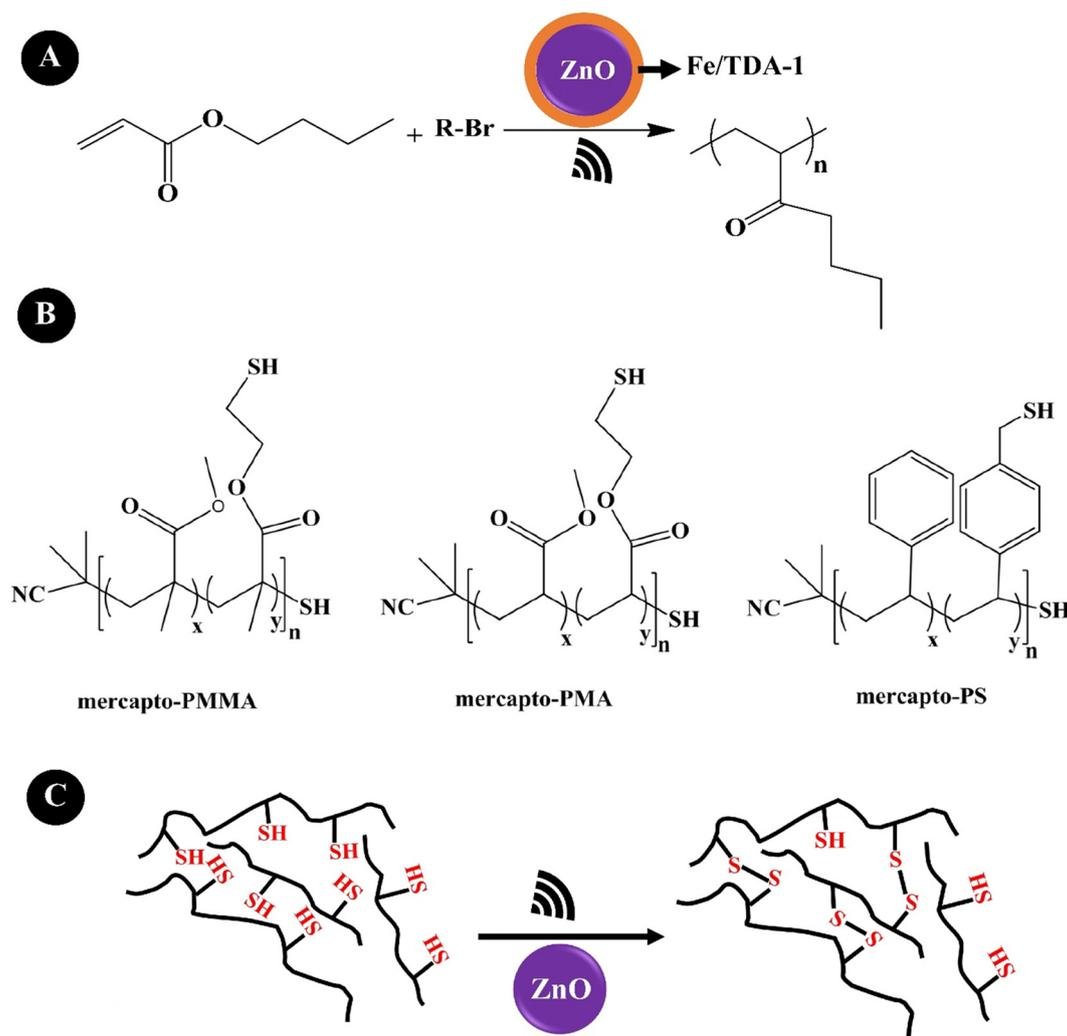
Fig. 9 The mechano-radical polymerization of acrylate monomers using ZnO NPs (A) (adapted from ref. 205 with permission from John Wiley and Sons). The chemical structures of mercapto-polymers (B) and mechanically promoted cross-linking of mercapto-polymers (C) (adapted from ref. 184 with permission from American Chemical Society).
