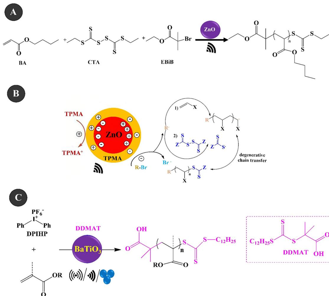
Fig. 7 The piezo-RAFT process (A) and mechanism (B) of BA (adapted from ref. 202 with permission from American Chemical Society). The piezo-RAFT polymerization of (meth)acrylate monomers over  $\text{BaTiO}_3$  under the three agitation conditions of US/BM/vortex (C) (adapted from ref. 203 with permission from John Wiley and Sons).
