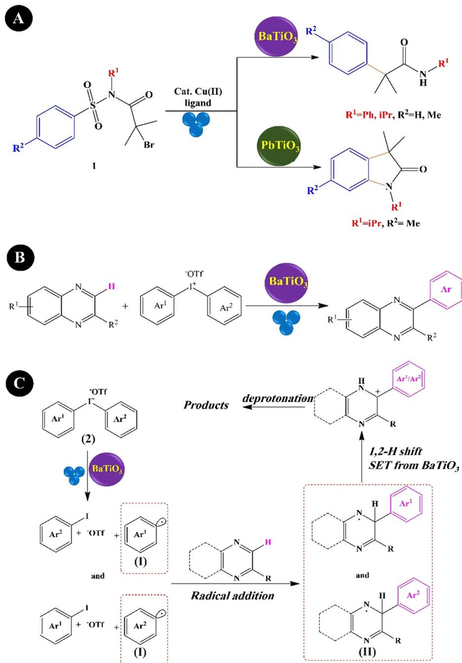
**Fig. 12** Mechano-induced synthesis of  $\alpha$ -arylamides and oxindoles (A) (adapted from ref. 214 with permission from John Wiley and Sons). The procedure (B) and mechanism (C) of mechano-induced C(sp<sup>2</sup>)-H arylation of quinoxalin(on)es (adapted from ref. 215 with permission from Elsevier).
