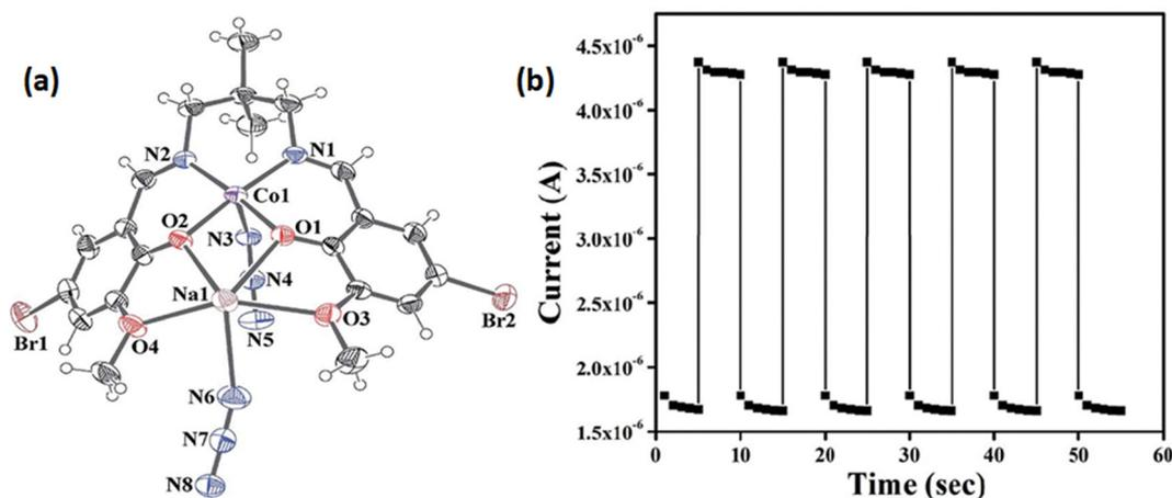
Fig. 4 (a) A thermal ellipsoid plot of a hetero-binuclear unit of **15** drawn with 40% ellipsoidal probability; (b) conductivity of the ITO/**15**/Al configuration under light-on and light-off conditions. Reproduced with permission from ref. 63. Copyright 2019 Royal Society of Chemistry.
