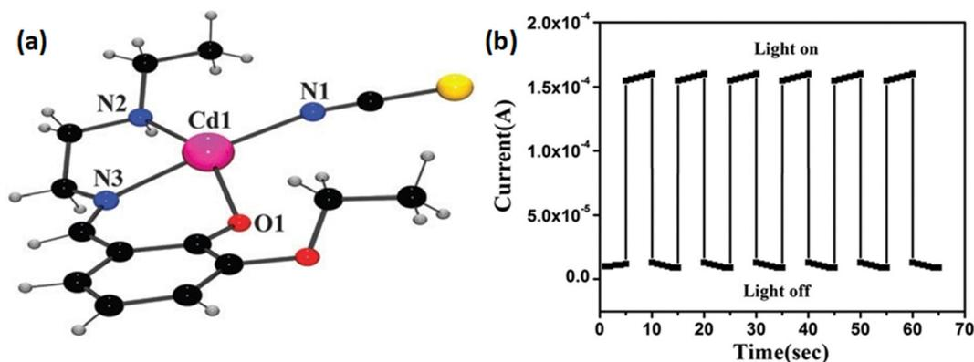
Fig. 2 (a) A perspective view of the asymmetric unit of **1**; (b) conductivity of ITO/**1**/Al configuration at light-on and light-off conditions. Reproduced with permission from ref. 53. Copyright 2015 Royal Society of Chemistry.
