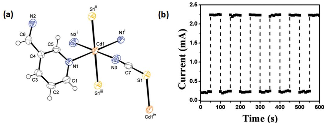
Fig. 3 (a) A thermal ellipsoid plot of an asymmetric unit of **2** drawn with 50% ellipsoidal probability; (b) conductivity of the device fabricated with **2** at light-on and light-off conditions (bias voltage = 1.0 V and intensity of incident light =  $80 \text{ mW cm}^{-2}$ ). Reproduced with permission from ref. 54. Copyright 2015 Royal Society of Chemistry.
