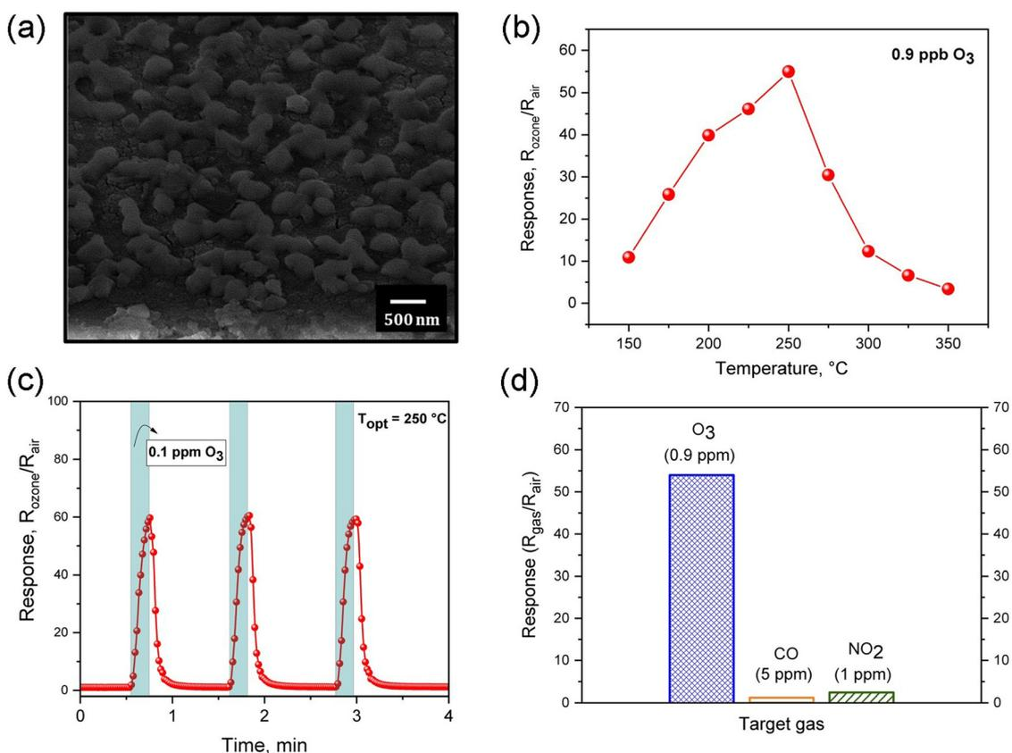
Fig. 6 ZnO thin film prepared *via* an RF-magnetron sputtering. (a) FESEM micrograph (b) sensing response at different operating temperatures, (c) dynamic response-recovery curves to 0.1 ppm of ozone, and (d) material selectivity towards different gas analytes.
