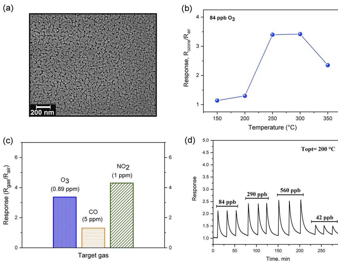
Fig. 5 Nanostructured ZnO thin film prepared *via* polymeric precursor method. (a) FESEM images (b) sensing response at different operating temperatures, (c) material selectivity towards different gas analytes, and (d) dynamic response-recovery curves as a function of the  $\text{O}_3$  gas level.
