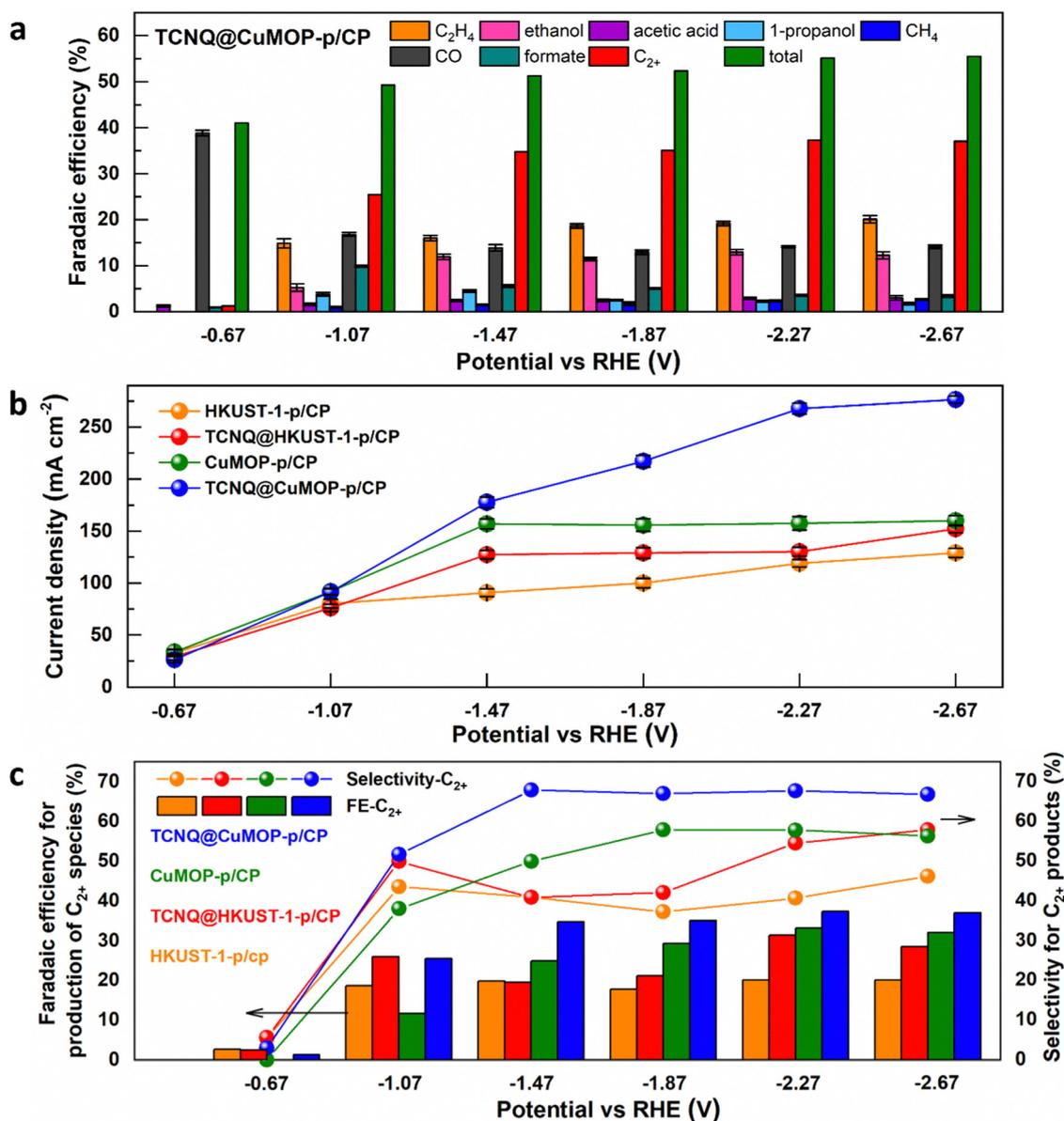
Fig. 4 (a) Catalytic performance of the TCNQ@CuMOP-p/CP electrode for  $\text{CO}_2\text{RR}$  at different potentials. (b) Comparison of the total current density over different electrodes for  $\text{CO}_2\text{RR}$  at different potentials. (c) Faradaic efficiency (FE) and selectivity to  $\text{C}_{2+}$  products over different electrodes for  $\text{CO}_2\text{RR}$  at different potentials.
