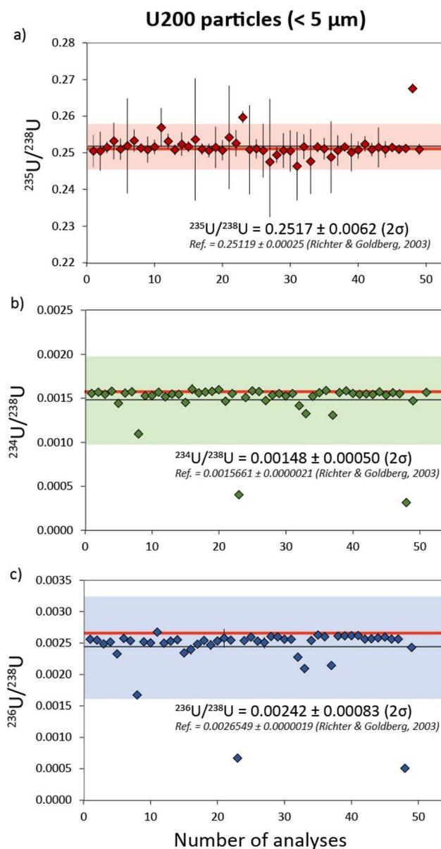
Fig. 3 Uranium isotope systematics for 49 separate U200 particles with  $^{235}\text{U}/^{238}\text{U}$ ,  $^{234}\text{U}/^{238}\text{U}$  and  $^{236}\text{U}/^{238}\text{U}$  data in (a), (b) and (c) respectively. Reference isotope ratios (red) are taken from Richter & Goldberg.<sup>16</sup> Uncertainties are  $2\sigma$ .
