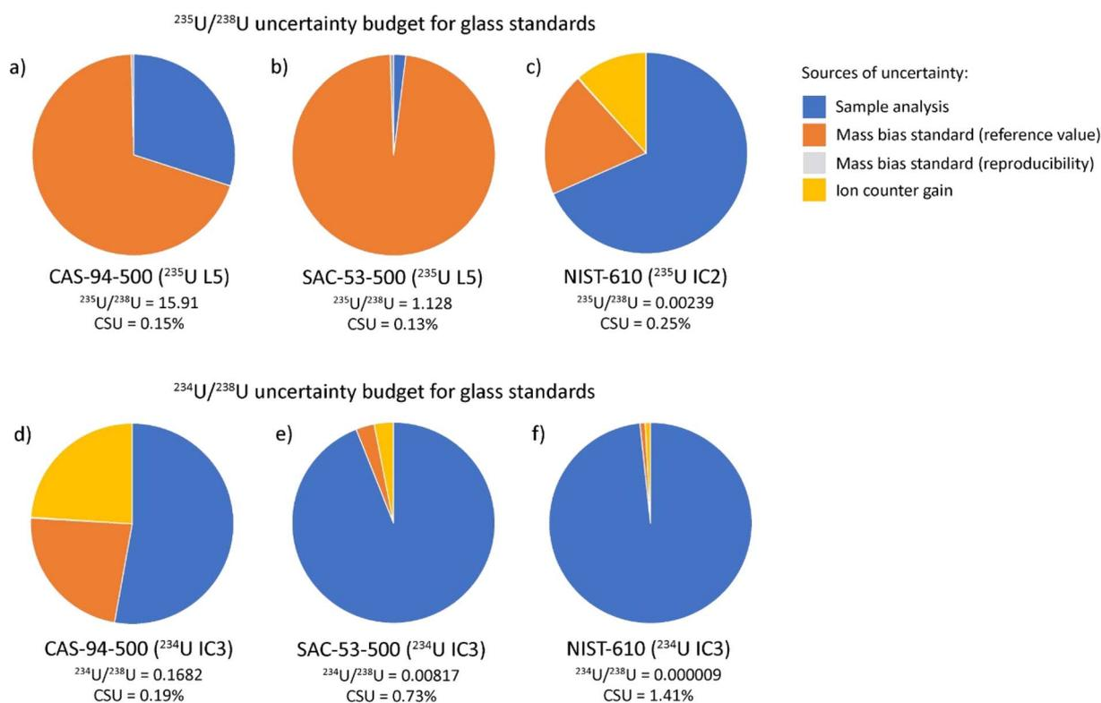
Fig. 2 Uranium isotope ratio uncertainty budgets for the three glass standards. The uncertainty budgets for  $^{235}\text{U}/^{238}\text{U}$  are provided in (a–c) and uncertainty budgets for  $^{234}\text{U}/^{238}\text{U}$  are provided in (d–f).
