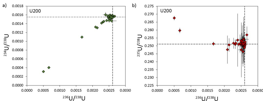
Fig. 4 Three isotope plots of the uranium composition in U200 particles with  $^{234}\text{U}/^{238}\text{U}$  vs.  $^{236}\text{U}/^{238}\text{U}$  in (a) and  $^{235}\text{U}/^{238}\text{U}$  vs.  $^{236}\text{U}/^{238}\text{U}$  in (b). Reference values (dashed lines) are from Richter & Goldberg.<sup>16</sup> All uncertainties are  $2\sigma$ .
