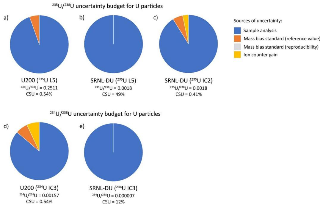
Fig. 8 Uranium isotope uncertainty budgets for the two U particle standards. The uncertainty budgets for  $^{235}\text{U}/^{238}\text{U}$  are provided in (a–c) and uncertainty budgets for  $^{234}\text{U}/^{238}\text{U}$  are provided in (d) and (e). The  $^{234}\text{U}/^{238}\text{U}$  uncertainty budget is largely representative of the budget for  $^{236}\text{U}/^{238}\text{U}$ .
