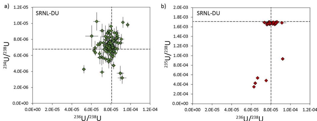
Fig. 7 Three isotope plots of the uranium composition in SRNL-DU particles with  $^{234}\text{U}/^{238}\text{U}$  vs.  $^{236}\text{U}/^{238}\text{U}$  in (a) and  $^{235}\text{U}/^{238}\text{U}$  vs.  $^{236}\text{U}/^{238}\text{U}$  in (b). Reference values (dashed lines) are from Scott *et al.*<sup>18</sup> All uncertainties are  $2\sigma$ .
