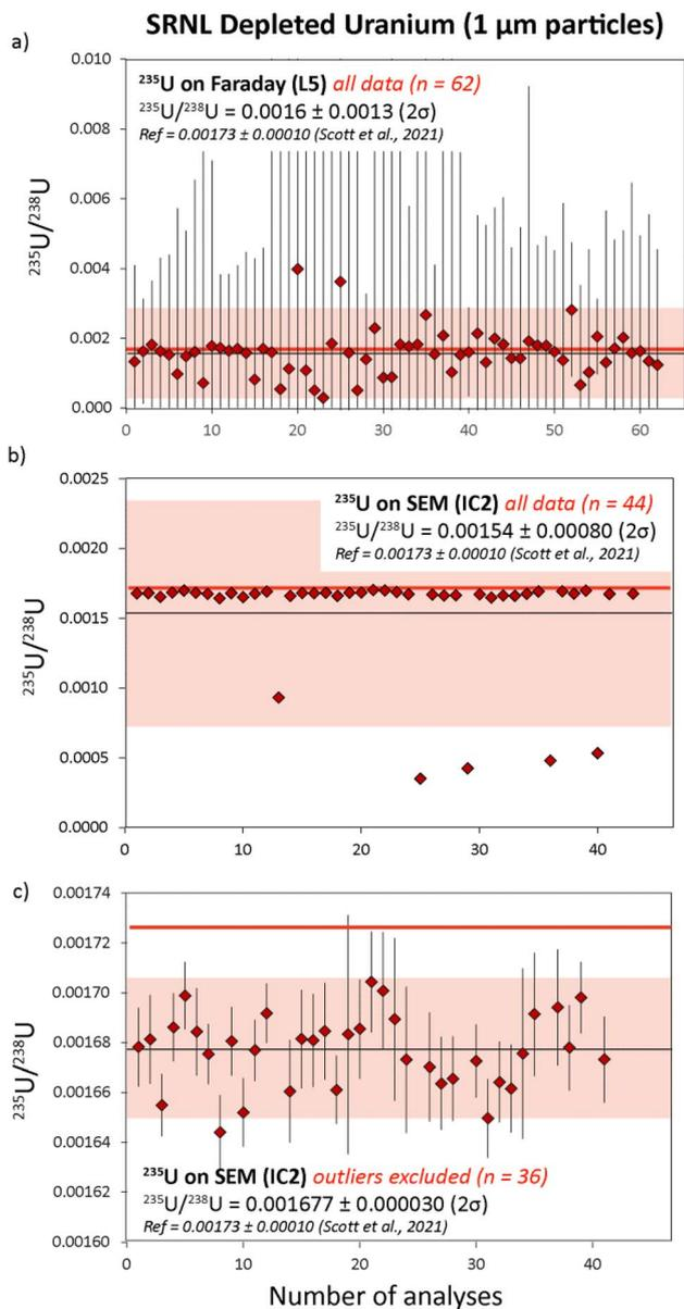
Fig. 5  $^{235}\text{U}/^{238}\text{U}$  ratios measured in SRNL-DU particles. In (a) the  $^{235}\text{U}$  was analyzed using the L5 Faraday. In (b) the  $^{235}\text{U}$  content was measured using IC2, and the final  $^{235}\text{U}/^{238}\text{U}$  average with five outliers excluded are in (c). Reference isotope ratios (red) are taken from Scott *et al.*<sup>18</sup> All uncertainties are  $2\sigma$ .
