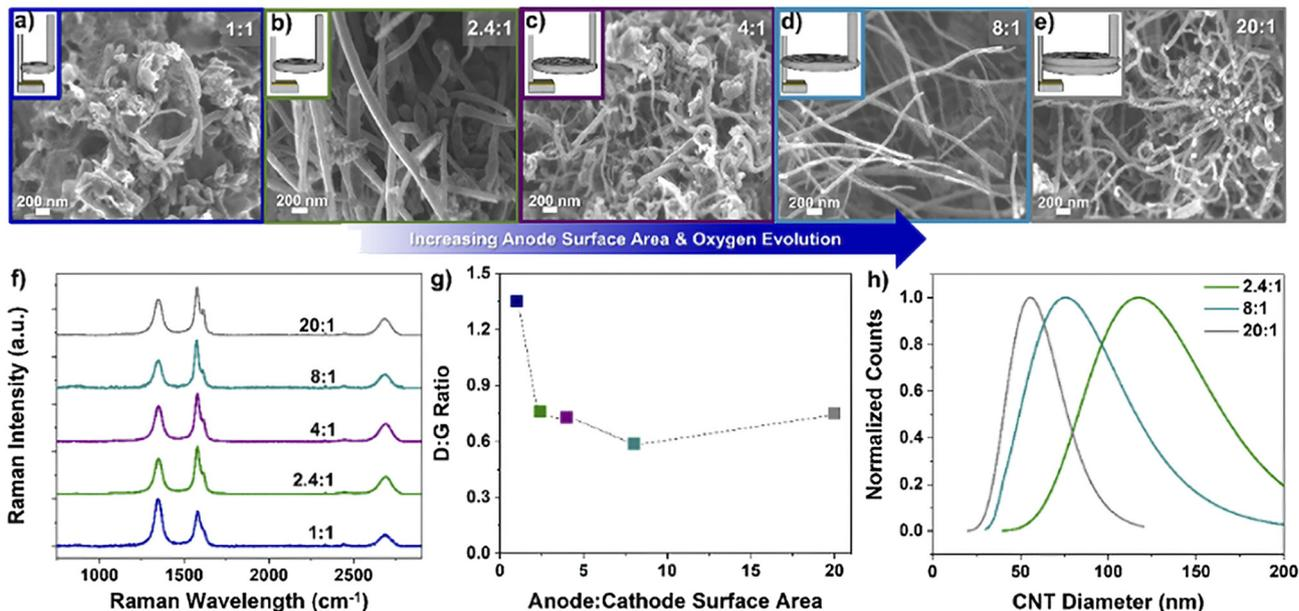
Fig. 12 Different anode to cathode surface area ratios (A : C) and the resulting carbon product using a Ni/Al<sub>2</sub>O<sub>3</sub> anode with 5 nm Fe on stainless steel cathode; a) 1 : 1, b) 2.4 : 1, c) 4 : 1, d) 8 : 1, e) 20 : 1 and f) Raman spectra, g) D : G ratio, and h) CNT diameter distribution at ratios of 2.4 : 1, 8 : 1, and 20 : 1.<sup>66</sup>
