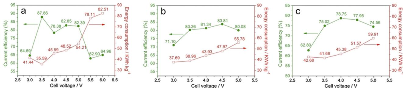
Fig. 15 Energy consumption and current efficiency under different cell voltages at 450 °C (a), 550 °C (b), and 650 °C (c).<sup>71</sup>
