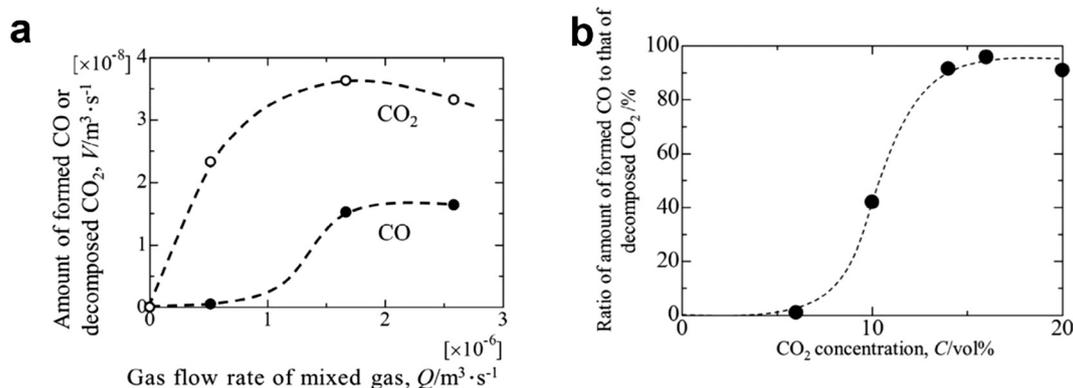
Fig. 16 (a) Amounts of decomposed CO<sub>2</sub> gas and produced CO gas as a function of inlet gas flow rate; (b) ratio of the amount of formed CO gas to that of decomposed CO<sub>2</sub> gas as a function of the initial gas concentration of CO<sub>2</sub>.<sup>42</sup>
