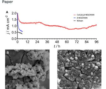
Fig. 5 (A) Long-term chronoamperometric ( $E=1.000\pm0.003~V~vs.$  SHE) AOR test of CoO $_x$ H $_y$ / $\beta$ -NiOOH/Ni (red) in 0.1 M K $_2$ HPO $_4+0.5~M$  NH $_3$ . Short-term (6 h) data for  $\beta$ -NiOOH/Ni (blue) and Ni foam (black) are shown for comparison. Currents are normalised to the geometric surface area of the electrodes (1 cm $^2$ ). (B and C) SEM images of the CoO $_x$ H $_y$ / $\beta$ -NiOOH/Ni electrode (B) as-prepared and (C) after the test shown in panel A.
