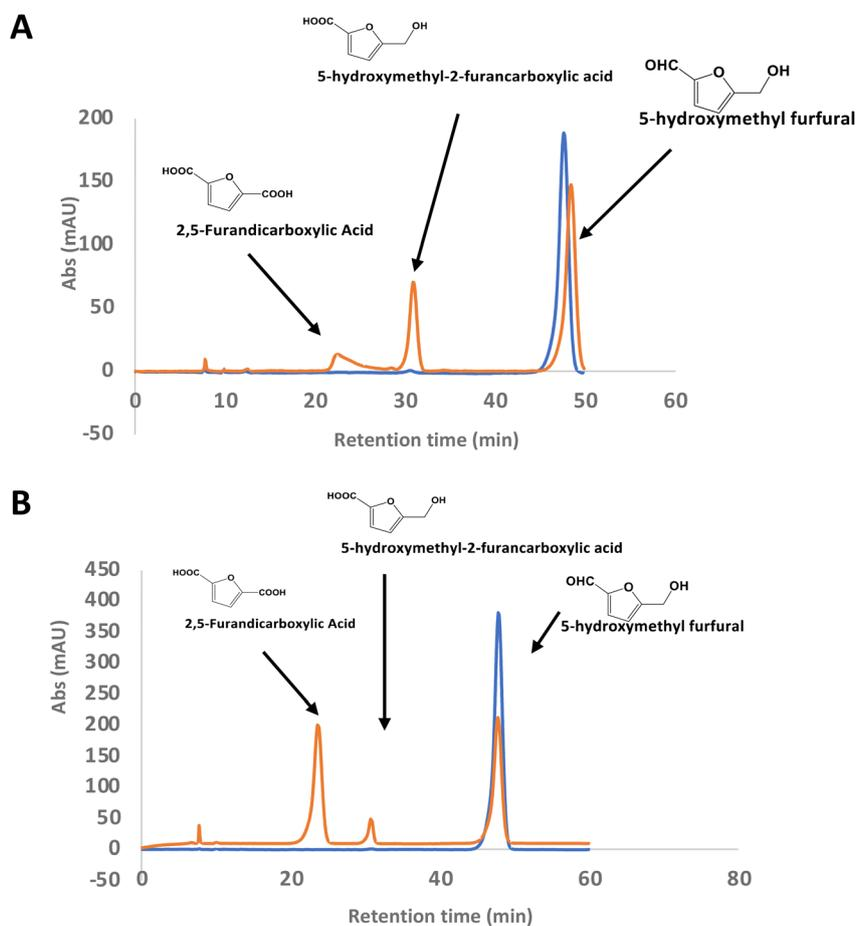
**Fig. 4** Conversion of HMF to FDCA by *R. jostii* RHA1 glycolate oxidase. (A) Small scale (1 ml) conversion of 2 mM HMF by 90  $\mu\text{g}$  Rj GLOx; (B) large scale (100 ml) conversion of 200 mg (16 mM) HMF by 9 mg Rj GLOx. Orange, reaction mixture containing enzyme; blue, control reaction lacking enzyme. All bioconversions incubated in 50 mM phosphate buffer pH 7.5 for 24 h at 30 °C.
