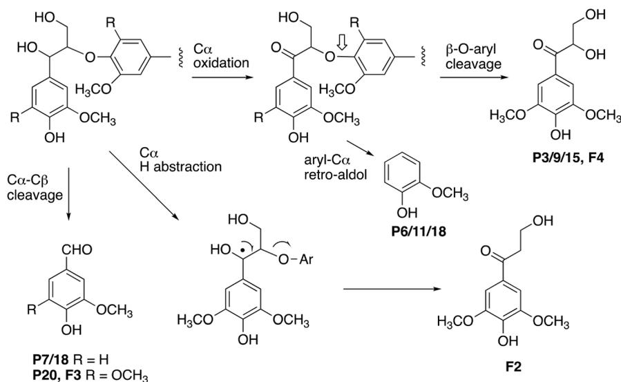
**Fig. 10** Formation of products from polymeric lignin. R = H (guaiacyl G lignin unit) or  $\text{OCH}_3$  (syringyl S lignin unit). Further oxidation of vanillin (P7/18) generates the corresponding carboxylic acid, vanillic acid (P2). Poplar organosolv lignin contains both S and G units (with proportion of S > G).
