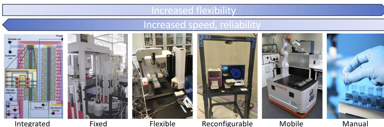
Fig. 2 Automation systems span a continuum of flexibility, speed, and reliability, from the integrated (e.g., as shown here, a microfluidic laboratory) to the fixed (e.g., Adam<sup>1</sup>), flexible (e.g., a bio workcell at Argonne), reconfigurable (e.g., a "cart" in Argonne's RPL), mobile (e.g., Liverpool's mobile robotic chemist<sup>6</sup>), and manual.
