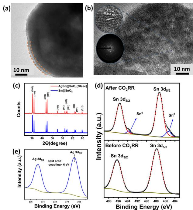
Fig. 2 (a) HRTEM image of AgSn@SnO<sub>x</sub> showing the thickness of the oxide layer, (b) *d*-spacing of the AgSn intermetallic phase and SAED pattern of AgSn@SnO<sub>x</sub> (30 s), (c) XRD patterns of Sn@SnO<sub>x</sub> and AgSn@SnO<sub>x</sub> (30 s), and (d) XPS patterns of AgSn@SnO<sub>x</sub> (30 s) before and after electrolysis depicting the Sn 3d spectrum, and (e) Ag 3d spectrum.
