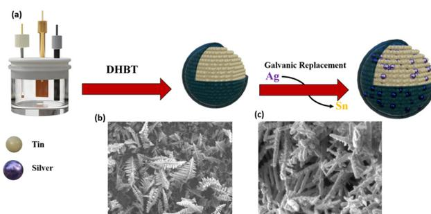
Fig. 1 (a) Synthesis steps of the AgSn@SnO<sub>x</sub> catalyst and (b) SEM images of Sn@SnO<sub>x</sub> and (c) AgSn@SnO<sub>x</sub> (30 s).
