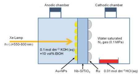
Fig. 14 Schematic of a plasmon-induced device for the photoelectrochemical synthesis of ammonia. Reproduced with permission from ref. 109. Copyright John Wiley & Sons.
