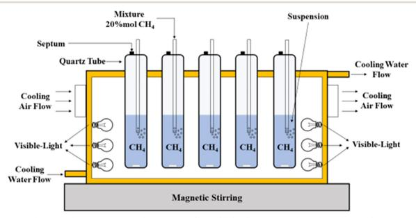
Fig. 7 Experimental setup for the photocatalytic partial oxidation of CH<sub>4</sub> to CH<sub>3</sub>OH. Reproduced with permission from ref. 81.
