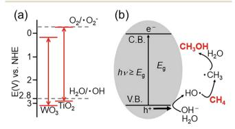
Fig. 9 Typical photocatalytic partial oxidation of methane to methanol mechanism catalyzed by metal oxide. (a) Redox potentials of WO<sub>3</sub> and TiO<sub>2</sub>. (b) Mechanism of the conversion of CH<sub>4</sub> to CH<sub>3</sub>OH by photocatalytic reaction. Adapted with permission from ref. 84 under the terms of the CC BY 3.0 license.
