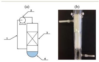
Fig. 15 The reactor diagram: (a) 1 - circulation loop; 2 - pump; 3 photocatalyst on a glass fiber cloth; 4 - water; (b) the quartz reactor bed. Reproduced with permission from ref. 125 under the terms of the CC BY license.
