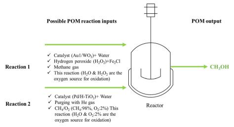
Fig. 8 Possible POM inputs with different reaction conditions
