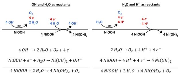
**Scheme 1** Decomposition pathways of NiOOH with H<sub>2</sub>O and OH<sup>−</sup> or H<sup>+</sup> as reactants. NiOOH catalyses the oxygen evolution reaction (OER), which provides the electrons for the Ni<sup>3+</sup> to Ni<sup>2+</sup> reduction. The protons for the phase transformation of NiOOH to Ni(OH)<sub>2</sub> are either delivered by the OER pathway as well or by the dissociation of H<sub>2</sub>O molecules.
