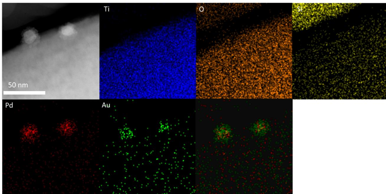
**Fig. 3** Microstructural analysis of the 0.33 wt% Au–0.33 wt% Pd/TS-1 catalyst including HAADF-STEM image and X-EDS mapping of the highlighted area showing the presence of AuPd nanoalloys with a Au-core Pd-shell morphology, Au (green), Pd (red), Ti (blue), and Si (yellow). Further analysis is reported in Fig. S3 and S4.†
