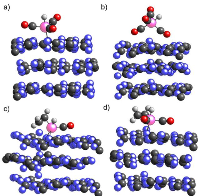
Fig. 5 Sketches of the optimized a)  $\text{H}_1\text{Rh}(\text{CO})_3$ , b)  $\text{H}_1\text{Rh}(\text{CO})_4$ , c)  $\text{H}_1\text{Rh}(\text{CO})(\text{C}_2\text{H}_4)$  and d)  $\text{H}_1\text{Rh}(\text{CO})_2(\text{C}_2\text{H}_4)$  species supported on ECN (grey, blue, pink, red, and white balls represent carbon, nitrogen, rhodium, oxygen, and hydrogen atoms respectively).
