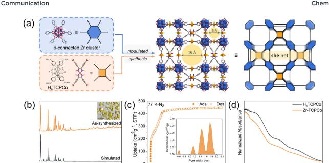
Fig. 1 (a) Schematic illustration of the design and synthesis of Zr-TCPCo with an **she** net; (b) PXRD patterns of Zr-TCPCo; inset: Optical micrograph of Zr-TCPCo; (c) 77 K  $N_2$  adsorption test of Zr-TCPCo; inset: diagram of incremental pore volume vs. pore width; (d) UV-vis spectra of Zr-TCPCo and the molecular cobaloxime  $H_4$ TCPCo.
