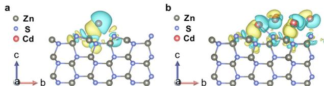
**Fig. 1** Charge transfer between low-work-function Cd and ZnS. The charge density difference of ZnS supported with Cd single atoms (a) and Cd clusters (b). The yellow and cyan contours around the atoms represent enriched and deficient electron clouds, respectively, which describes the charge transfer of the ZnS support after contacting Cd single atoms and clusters, respectively.
