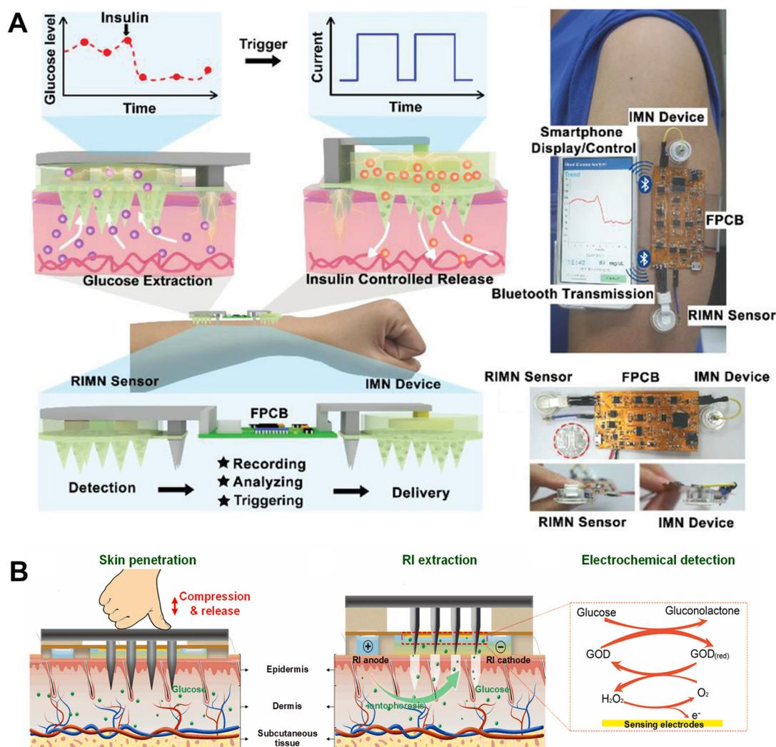
**Fig. 5** ISF collection by iontophoresis through porous and solid MNs. (A) A closed-loop system based on mesoporous MN-RI for diabetes treatment. Adapted with permission from ref. 75. Copyright 2021, Wiley-VCH. (B) A touch-actuated glucose sensor fully integrated with solid MNs and RI for diabetes monitoring. Adapted with permission from ref. 22. Copyright 2022, Elsevier.
