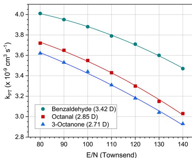
**Fig. 10** Dependence of the proton-transfer reaction constant  $k_{\text{PT}}$  on the  $E/N$  ratio (electric field to molecular density) set in the PTR-MS device at 353 K for benzaldehyde, octanal and 3-octanone. The values in brackets indicate the respective dipole moment in Debye. The data were taken from Salthammer *et al.*<sup>135</sup>
