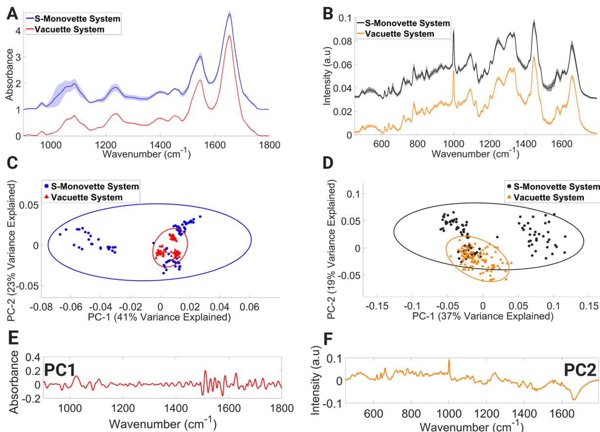
**Fig. 2** Mean FTIR (A) and Raman (B) spectra of lymphocytes collected with S-Monovette® or Vacuette® blood collection systems, PCA score plot of FTIR (C) and Raman (D) spectra, PC1 loading of FTIR spectra (E) and PC2 loading of Raman spectra (F). Covariance ellipses (95% confidence limit) in (C) and (D) are shown for each data class.
