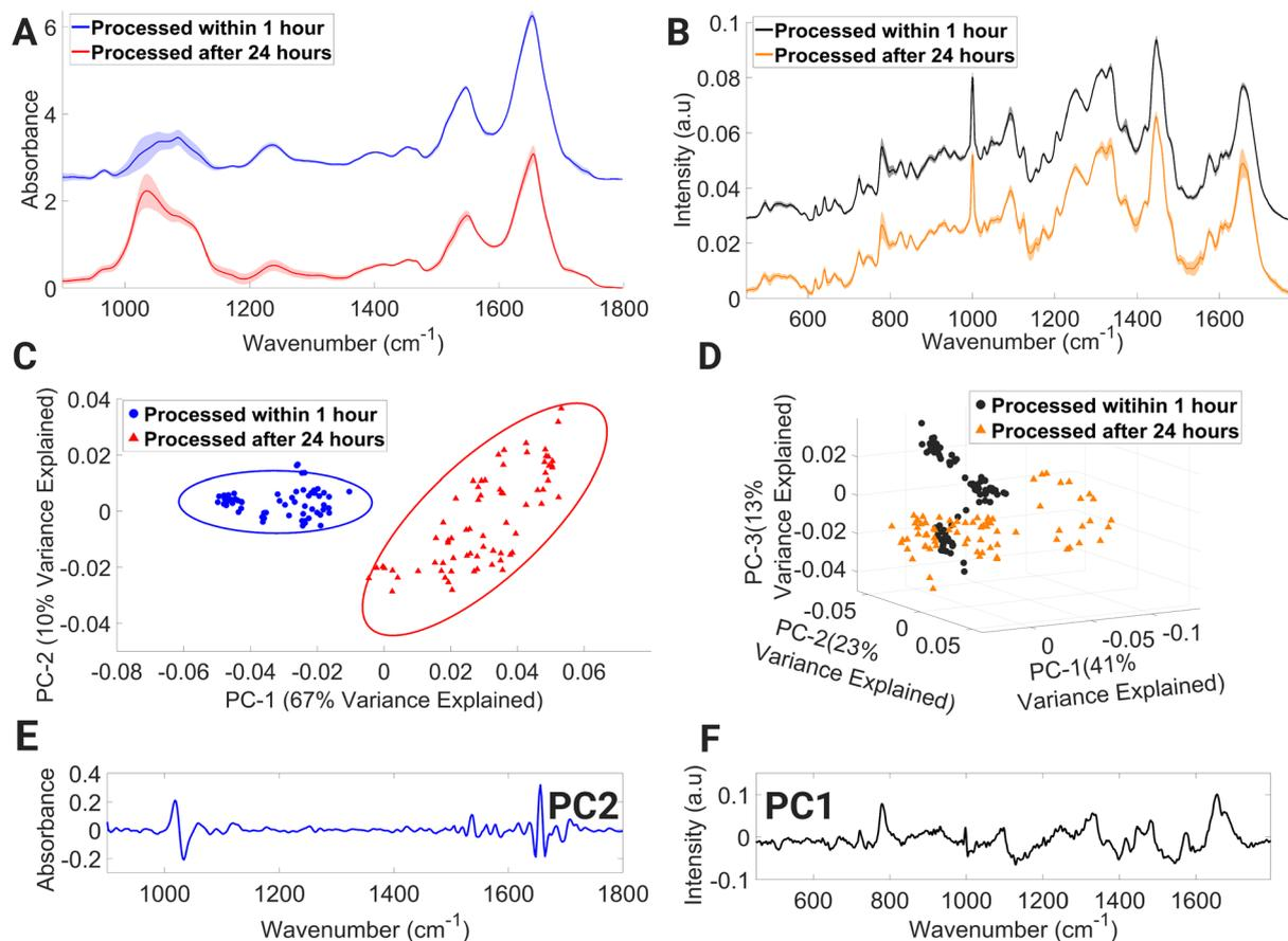
**Fig. 7** Mean FTIR (A) and Raman (B) spectra of lymphocytes processed immediately and 24 hours after collection, PCA score plot of FTIR (C) and Raman (D) spectra, PC2 loading of FTIR spectra (E), PC1 loading of Raman spectra (F). Covariance ellipses (95% confidence limit) in (C) are shown for each data class.
