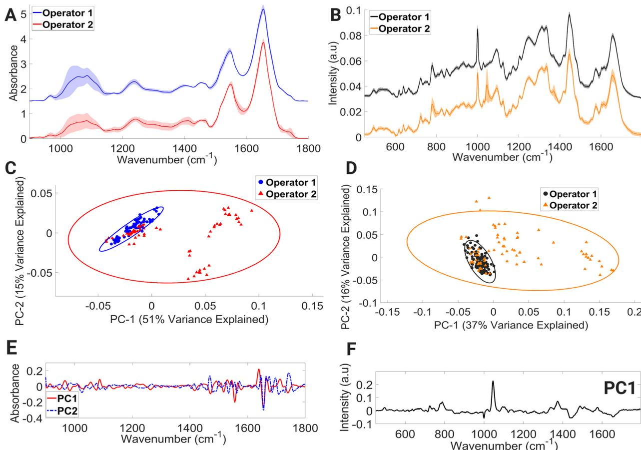
**Fig. 6** Mean FTIR (A) and Raman (B) spectra of lymphocytes processed by operator 1 and 2, PCA score plot of FTIR (C) and Raman (D) spectra, PC1 and PC2 loading of FTIR spectra (E), PC1 loading of Raman spectra (F). Covariance ellipses (95% confidence limit) in (C) are shown for each data class.
