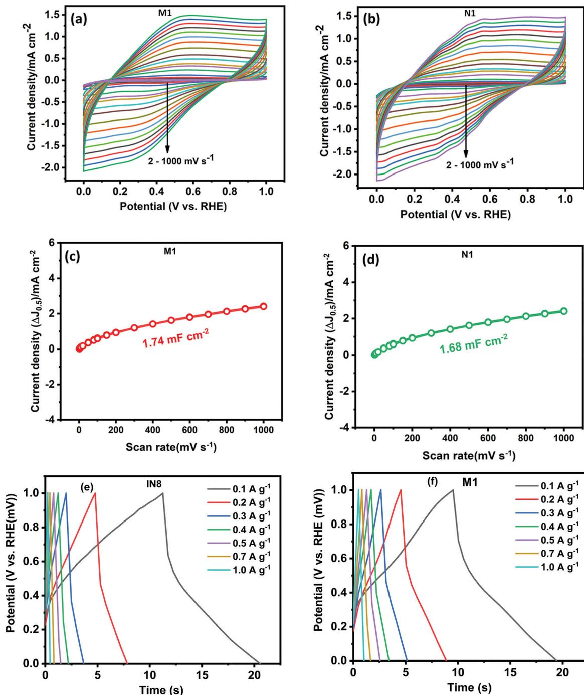
Fig. 7 CV curves at various scan rates of (a) N1 and (b) M1; graphs showing current density ( $\Delta j_{0.5}$ ) vs scan rate of (c) M1 and (d) N1; GCD curves of (e) N1 and (f) M1.
