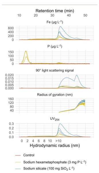
Fig. 2 Fractograms representing triplicate sodium silicate and hexametaphosphate suspensions and a control suspension (no sequestrant). Theoretical hydrodynamic radius was calculated at constant crossflow ( $\leq$ 31 min retention time), based on channel geometry and flow parameters.<sup>32</sup> Light scattering and absorbance fractograms are displayed with the raw detector responses on the *y*-axis.
