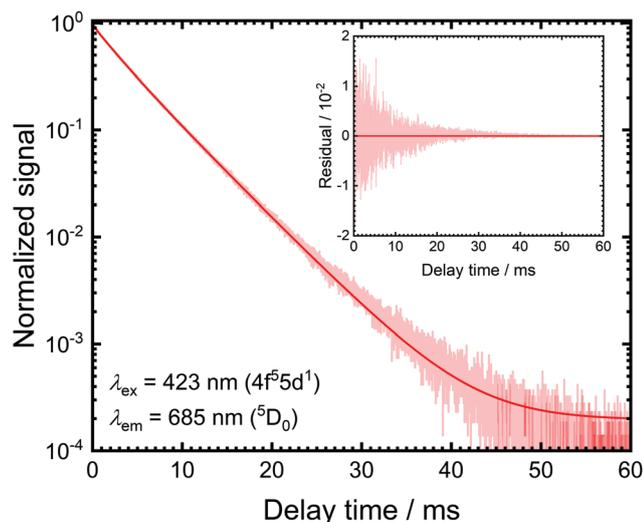
Fig. 2 The photoluminescence decay curve recorded upon monitoring the  ${}^5D_0 \rightarrow {}^7F_0$  transition at 685 nm ( $\lambda_{\text{ex}} = 423$  nm) at room temperature. The solid red line indicates a single exponential fit and the inset depicts the respective residual plot.
