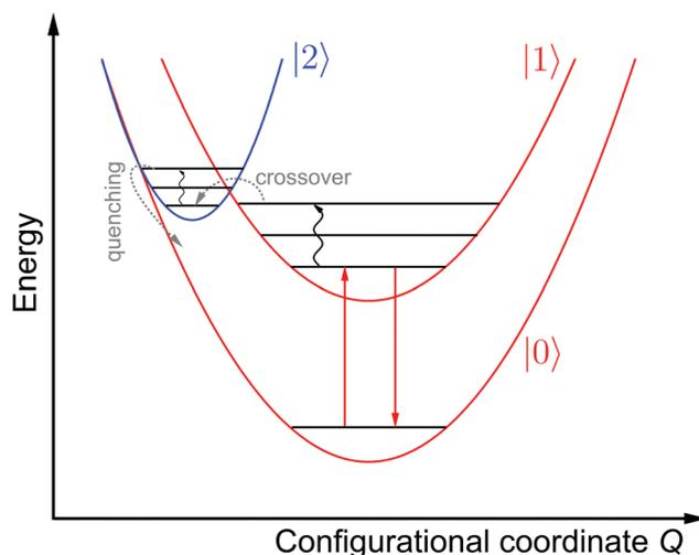
Fig. 3 Schematic overview of the different processes determining the performance of a luminescent crossover thermometer such as  $\text{Sm}^{2+}$ . Curvy arrows indicate (multi-)phonon absorption transitions. Note that the excited state  $|2\rangle$  has been depicted at lower configurational coordinates to match the theoretical and experimental findings for low excited  $4f^{n-1} 5d^1$  states of lanthanoid ions (see also text).
