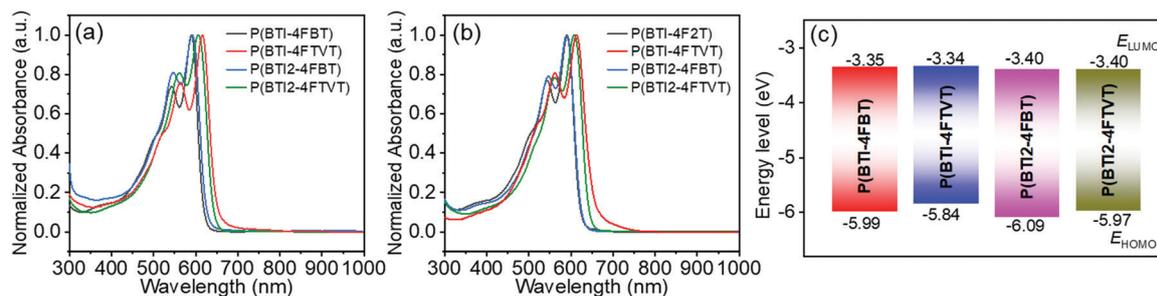
**Fig. 3** (a) Solution and (b) thin-film UV-vis-NIR absorption spectra and (c) energy level diagrams of the polymers. Solution spectra were measured in *o*-DCB with a concentration of  $10^{-5}$  mol L $^{-1}$  of the repeating units. Thin films were prepared by spin-coating the *o*-DCB solutions on quartz substrates.  $E_{\text{HOMO}}$  and  $E_{\text{LUMO}}$  values were estimated from the redox onsets in the thin-film cyclic voltammetry curves.
