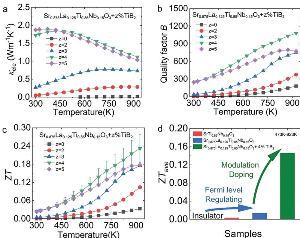
Fig. 10 Thermal transport properties of  $\text{Sr}_{0.875}\text{La}_{0.125}\text{Ti}_{0.85}\text{Nb}_{0.15}\text{O}_3 + z\% \text{ TiB}_2$  ( $z = 0-5$ ): (a)  $\sigma$ ; (b) quality factor B; (c) ZT; and (d) average ZT of  $\text{SrTi}_{0.85}\text{Nb}_{0.15}\text{O}_3$ ,  $\text{Sr}_{0.875}\text{La}_{0.125}\text{Ti}_{0.85}\text{Nb}_{0.15}\text{O}_3$  and  $\text{Sr}_{0.875}\text{La}_{0.125}\text{Ti}_{0.85}\text{Nb}_{0.15}\text{O}_3 + 4\% \text{ TiB}_2$ .
