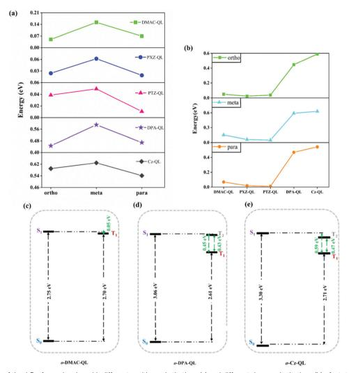
Fig. 4 Comparison of the  $\Delta E_{ST}$  for molecules with different position substitutions (a) and different donor substitutions (b) of a total of 15 molecules in tetrahydrofuran ( $\Delta E_{ST} = S_1 - T_1$ ). Adiabatic excitation energies for o-DMAC-QL (c), o-DPA-QL (d) and o-Cz-QL (e) in tetrahydrofuran, respectively.
