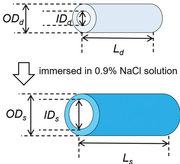
**Scheme 1** Illustration of the dimensional changes test. The dimensional changes of the inner diameter (I.D.), outer diameter (O.D.), and length were expressed as  $ID_s/ID_d$ ,  $OD_s/OD_d$ , and  $L_s/L_d$ , respectively.
