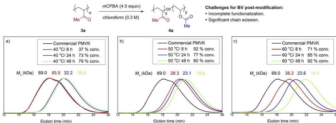
Fig. 1 The influence of temperature and reaction time on the BV oxidation of PMVK in chloroform. SEC traces of commercial PMVK **3a** before and after BV oxidation at (a) 40 °C, (b) 50 °C and (c) 60 °C with different reaction time.
