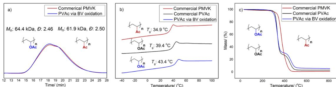
Fig. 4 Characterization of PVAc **5a** prepared by exhaustive BV post-modification of PMVK **3a**. Comparison of (a) SEC, (b) DSC, and (c) TGA data of PMVK **3a**, commercial PVAc and PVAc **5a** obtained by BV oxidation.
