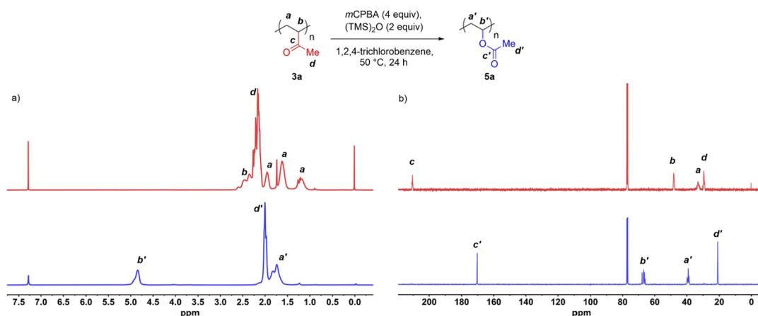
Fig. 3 Exhaustive BV oxidation of commercial PMVK homopolymers. Comparison of (a)  $^1\text{H}$  NMR spectra and (b)  $^{13}\text{C}$  NMR spectra before and after exhaustive BV oxidation of commercial PMVK **3a**. The NMR spectra were recorded using  $\text{CDCl}_3$  as a solvent.
