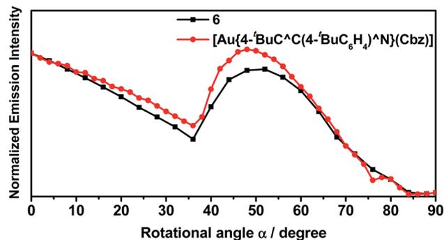
Fig. 6 Angular-dependent PL intensities of the p-polarized light of **6** and  $[\text{Au}\{4\text{-}^t\text{BuC}^{\wedge}\text{C}(4\text{-}^t\text{BuC}_6\text{H}_4)^{\wedge}\text{N}\}(\text{Cbz})]$  (11% v/v) in *m*-CBP thin films with 20 nm thickness.
