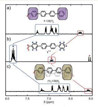
Fig. 2 Supramolecular complexation of  $1^{2+}$  and CB[n].  $^1$ H NMR spectra of  $1^{2+}$  at (a)  $\chi_{\text{CB[7]}}=2$ , (b)  $\chi_{\text{CB[}n]}=0$  and (c)  $\chi_{\text{CB[8]}}=1$  in D<sub>2</sub>O. Cl $^-$  counter-ions are omitted for clarity.
