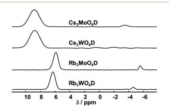
Fig. 3  $\,^{2}$ H MAS NMR spectra of the four compounds (isotropic region only). The spectra were acquired at room temperature with a spinning frequency of 5 kHz and a magnetic field  $B_{0}=17.6$  T.
