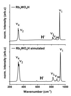
Fig. 4 Experimental Raman spectrum of  $Rb_3WO_4H$  (top) and simulated Raman spectrum of  $Rb_3WO_4H$  (bottom, DFT-PBE0 method).
