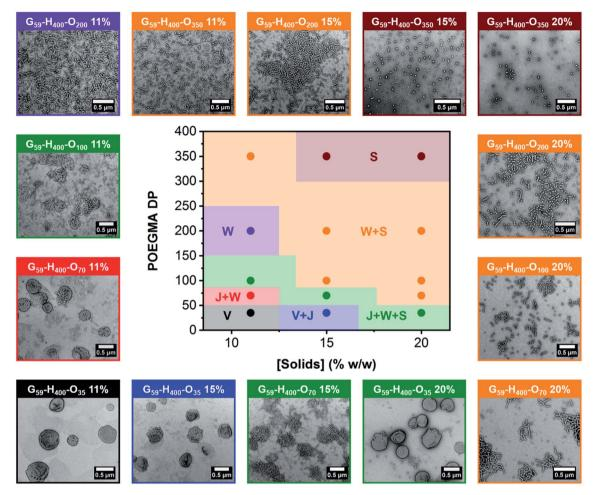
Fig. 3 Pseudo-phase diagram constructed for  $G_{59}$ - $H_{400}$ - $O_x$  triblock copolymer nano-objects (x=35-350) prepared via RAFT-mediated aqueous PIDA by systematically varying the total solids content and target POEGMA DP. Representative TEM images obtained using a 0.75% w/w uranyl formate staining solution are shown for each formulation. Each frame color corresponds to a different nano-object morphology (S = spherical micelles; W = worms; J = jellyfish and V = vesicles).
