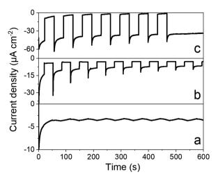
Fig. 6 Photocurrent densities measured under chopped visible light  $(400 < \lambda < 800 \text{ nm}, 65 \text{ mW cm}^{-2})$  at an applied potential of 0.065 V vs. RHE in 0.1 M acetate buffer (pH 4.5) for the following electrodes: FTO/ NiO (a), FTO/NiO/P3HT:PCBM (b) and FTO/NiO/[P3HT:PCBM+1] (c).
