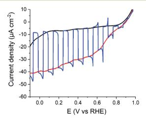
Fig. 5 LSVs at FTO/NiO/[P3HT:PCBM+1] electrode with (red line), without (black line) or with chopped (blue line) visible light (400 <  $\lambda$  < 800 nm, 65 mW cm<sup>-2</sup>) recorded at a scan rate of 5 mV s<sup>-1</sup> in 0.1 M acetate buffer (pH 4.5).
