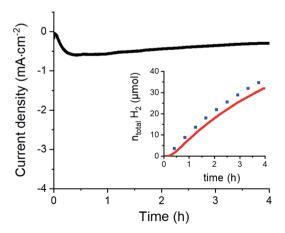
Fig. 4 Long-term chronoamperometric experiment at -0.63 V vs. RHE in acetate buffer (0.1 M, pH 4.5) with concomitant H<sub>2</sub> quantification (red trace in inset); the blue dots indicate the expected H<sub>2</sub> amount for a 100% faradaic yield.
