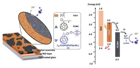
Fig. 1 Representation (left) and energy diagram (right) of a photocathode for  $H_2$  evolution based on a PCBM:P3HT bulk heterojunction BHJ combined with the cobalt diimine-dioxime – fullerene assembly 1 as  $H_2$ -evolving catalyst (see ESI† and ref. 30 for energy values).
