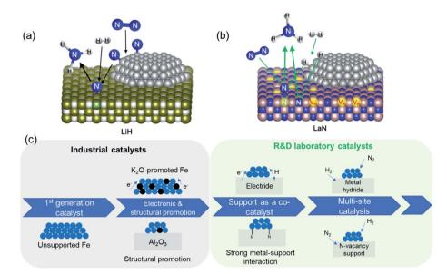
Fig. 3 (a) Schematic of multi-site reaction mechanism over transition metal-loaded LiH; reproduced from ref. 84 with permission from Springer Nature, copyright 2020; (b) schematic of Mars-van Krevelen reaction mechanism over transition metal-loaded LaN; reproduced from ref. 84 with permission from Springer Nature, copyright 2020; (c) evolution in the complexity of heterogeneous catalyst design for ammonia synthesis: from a simple metal surface to multi-site approaches.
