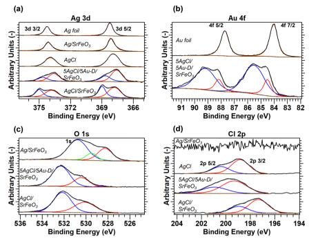
Fig. 4 XPS spectra for (a) Ag 3d, (b) Au 4f, (c) Cl 2p, and (d) O 1s scans, with deconvoluted peaks fitted to experimental measurements. Measurements calibrated with respect to Au 4f<sub>7/2</sub> peak at BE = 84.0 eV. Full details of peak deconvolution are given in the ESI,† Table S4.
