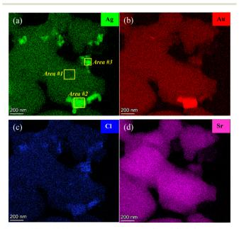
Fig. 3 STEM-EDS maps of crushed 5Ag/5Au-D/SrFeO<sub>3</sub> particles, showing distribution of (a) Ag, (b) Au, (c) Cl, (d) Sr. Area 1 corresponds to bare SrFeO<sub>3</sub> support with no Ag or Au detected, Area 2 corresponds to a particle of AgAu, Area 3 corresponds to a particle of AgCl.
