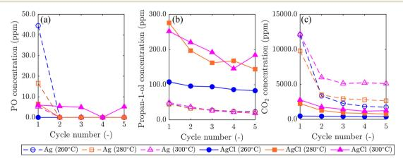
Fig. 8 Graphs showing comparison of reaction products: (a) PO, (b) propan-1-ol, and (c) CO<sub>2</sub> in experiments over Ag/SrFeO<sub>3</sub> and AgCl/SrFeO<sub>3</sub>, in the temperature range 260-300 °C. Lines between cycles included to help differentiate samples.
