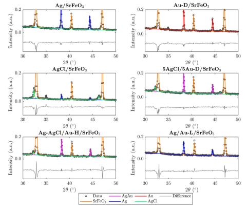
Fig. 2 Sections of collected XRD patterns for Ag/SrFeO<sub>3</sub>, Au-D/SrFeO<sub>3</sub>, AgCl/SrFeO<sub>3</sub>, 5AgCl/5Au-D/SrFeO<sub>3</sub>, Ag-AgCl/Au-H/SrFeO<sub>3</sub>, and Ag/Au-L/ SrFeO<sub>3</sub>. Circles indicate experimental measurements; lines indicate fitted model using reference patterns.
