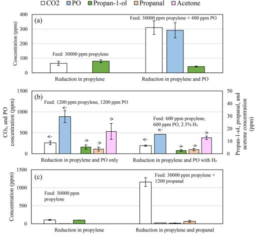
Fig. 11 Reaction products for reaction over 5Ag/5Au-D/SrFeO<sub>3</sub>, for (a) propylene with and without PO added (b) dilute PO/propylene, with and without H<sub>2</sub> (c) for propylene with and without propanal added. Error bars show standard deviation from 3 cycles, arrows indicate y-axis for each species. Feed composition given on each figure, with balance gas Ar/N<sub>2</sub>.
