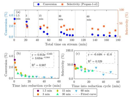
Fig. 6 Chemical looping over 7.5AgCl/2.5Au-D/SrFeO<sub>3</sub>, with reduction time increased from 1.5 to 60 min. Vertical dotted lines in (a) indicate start and end of each reduction step. Change in conversion of propylene (b), and in selectivity towards propan-1-ol (c).
