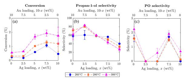
Fig. 7 Graphs showing average values of (a) propylene conversion, (b) selectivity towards propan-1-ol, and (c) selectivity towards PO, for xAqCl/ (10-x)Au-D/SrFeO<sub>3</sub> samples (x = 0, 2.5, 5, 7.5, 10). Error bars show standard deviation over 5 cycles, noting that some error bars are smaller than the datapoint markers. Sample at x = 0 corresponds to Au-D/SrFeO<sub>3</sub>; sample at x = 10 corresponds to AgCl/SrFeO<sub>3</sub>.
