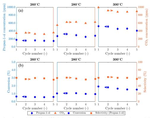
Fig. 5 (a) Concentrations of propan-1-ol and CO<sub>2</sub> and (b) calculated propylene conversion and selectivity towards propan-1-ol (shown on left and right axes, respectively) over the temperature range 260-300 °C for 5AgCl/5Au-D/SrFeO<sub>3</sub>.
