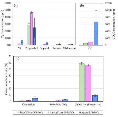
Fig. 9 Comparison of (a) concentrations of C<sub>3</sub> products, (b) concentrations of CO<sub>2</sub>, and (c) overall conversion and selectivity, for 5AqCl/5Au-D/ SrFeO<sub>3</sub>, Ag-AgCl/Au-H/SrFeO<sub>3</sub>, and Ag/Au-L/SrFeO<sub>3</sub> at 280 °C. Error bars correspond to standard deviation over 5 cycles.
