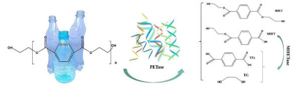
Fig. 10 PETase degradation process of PET.
