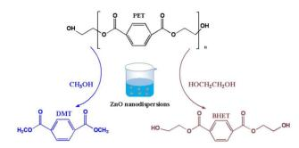
Fig. 11 Nano-ZnO dispersion catalyzed depolymerization of PET.
