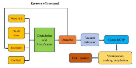
Fig. 13 DOTP made from waste PET.
