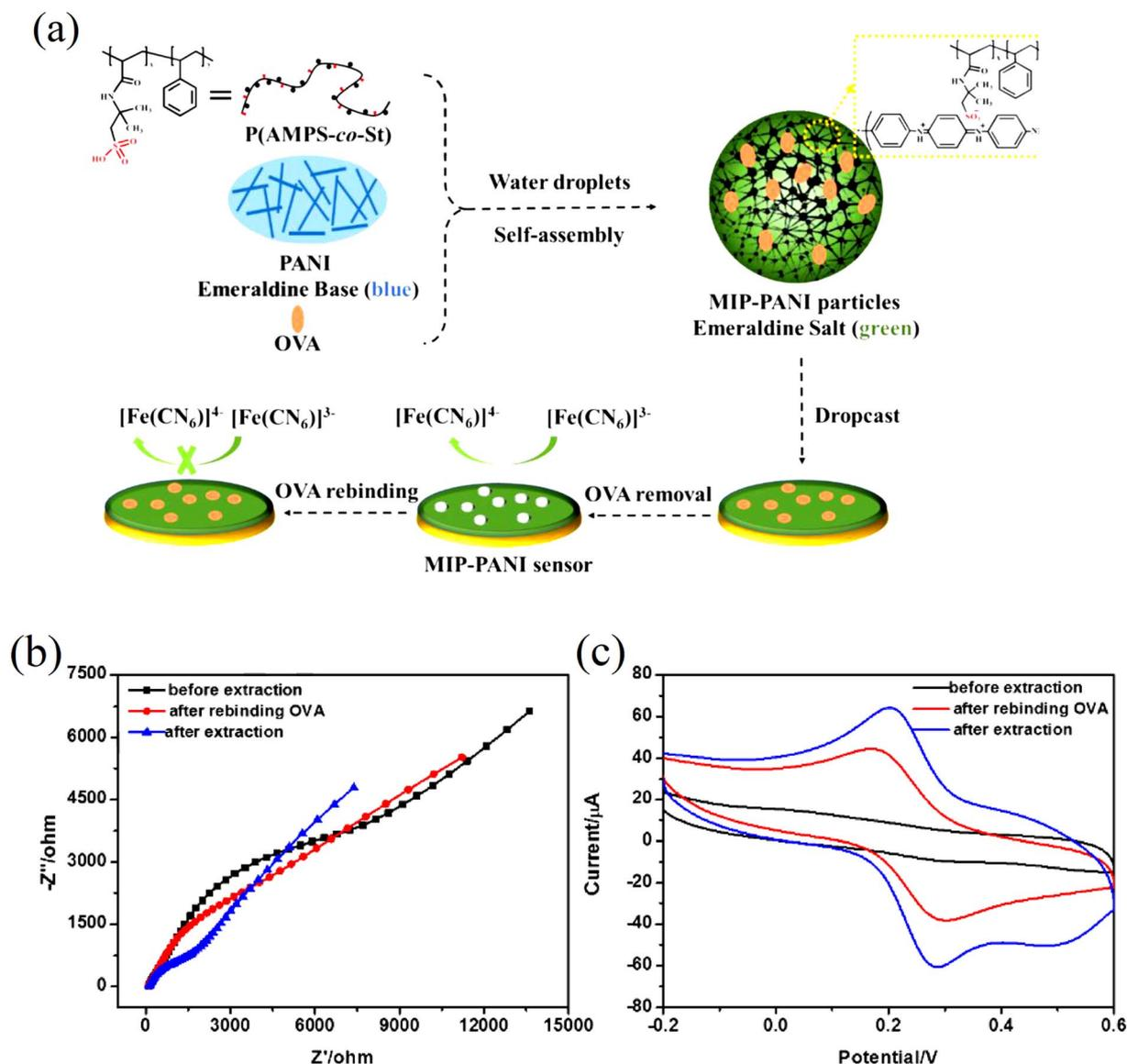
Fig. 3 (a) Schematic illustration of the synthesis of MIP-PANI particles and the fabrication of MIP-PANI sensor, (b) EIS curves and (c) CV curves of MIP-PANI particles modified electrode in  $[\text{Fe}(\text{CN})_6]^{3-/4-}$  solution before extraction, after extraction and after rebinding OVA by incubation in  $0.5 \text{ mg mL}^{-1}$  OVA solution (reprinted with permission from Elsevier, ref. 21 Luo *et al.*, (2017)).
