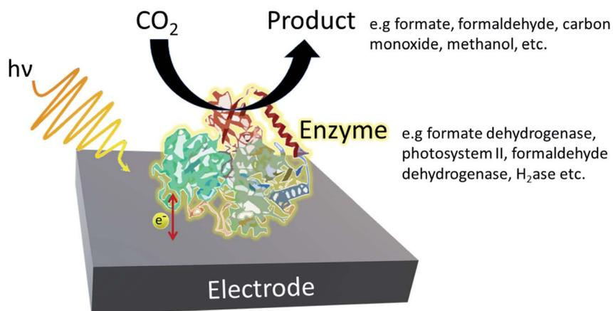
Fig. 3 Example of a typical enzymatic photohybrid system in which CO<sub>2</sub> is reduced by the enzyme to produce the appropriate biofuel.
