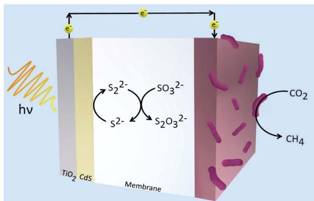
Fig. 4 Hybrid microbial photosystem designed by Xiao *et al.* consisting of a TiO<sub>2</sub>/CdS photoanode and a biocathode for CO<sub>2</sub> reduction to CH<sub>4</sub>.<sup>106</sup> The sulfide electrolyte solution was used as sacrificial reagents to consume holes and prevent the corrosion of CdS.
