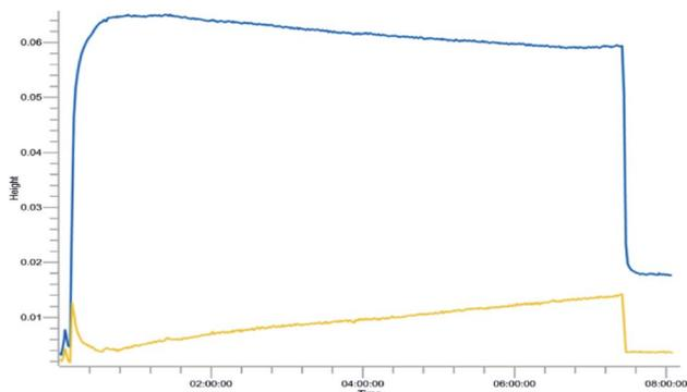
Fig. 6 Trend analysis of furfural reduction for the scale-up reduction. Wavenumbers selected: 1713  $\text{cm}^{-1}$  (blue) to acetone and 1680  $\text{cm}^{-1}$  (yellow) for the aldehyde. Reaction conditions: a 0.25 M solution of furfural in iso-propanol was pumped through a BZC column at 120 °C and 50 s residence time for 5.5 hours.
