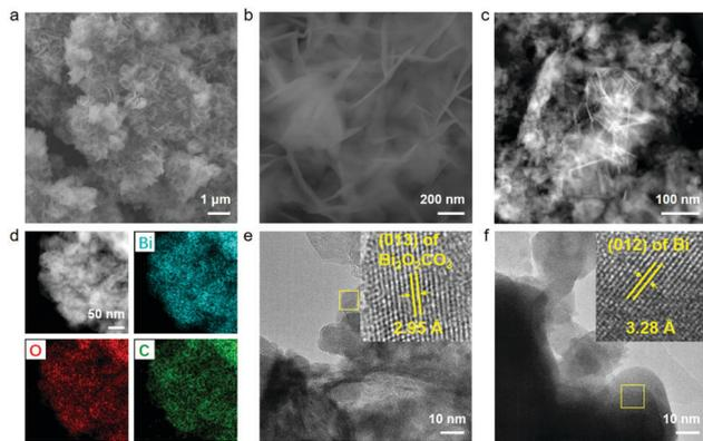
Fig. 3 (a and b) SEM, (c) TEM and (d) STEM-EDS elemental maps of VS-Bi<sub>2</sub>O<sub>3</sub> after the CO<sub>2</sub>RR for 10 h. (e and f) HR-TEM images of VS-Bi<sub>2</sub>O<sub>3</sub> after the CO<sub>2</sub>RR for 10 h in which Bi<sub>2</sub>O<sub>2</sub>CO<sub>3</sub> and metallic Bi are detected *via* their characteristic facets.
