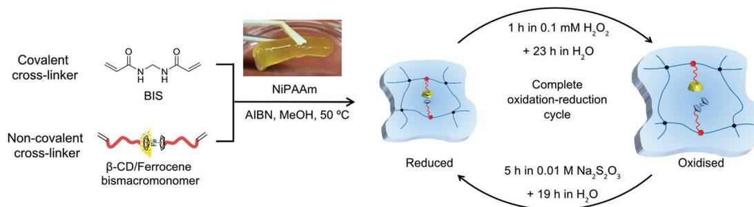
**Fig. 4** Chemical structure and synthesis steps of supramolecular redox responsive ferrocene- $\beta$ -CD hydrogels, including the optimised procedure to achieve fully oxidised and fully reduced hydrogels.
