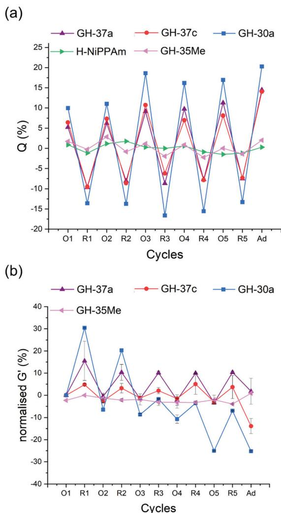
**Fig. 6** (a) Swelling degree and (b) normalised storage modulus of supramolecular hydrogels GH-37a, GH-37c, GH-30a and control hydrogels H-PNiPAAm and GH-35Me. R1–R5 and O1–O5 correspond to the cycle number of reduction and oxidation, respectively.
