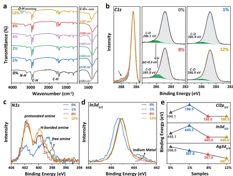
Fig. 3 (a) FTIR spectra, XPS spectra of (b) C 1s, (c) N 1s, and (d) In 3d core levels, and (e) a summary of changes on the XPS peaks of Cl 2p, In 3d, and Ag 3d core levels of  $\text{Cs}_2\text{AgInCl}_6$ :x% Te,1% Bi NCs ( $x = 0, 1, 2, 4, 8, 12$ ).
